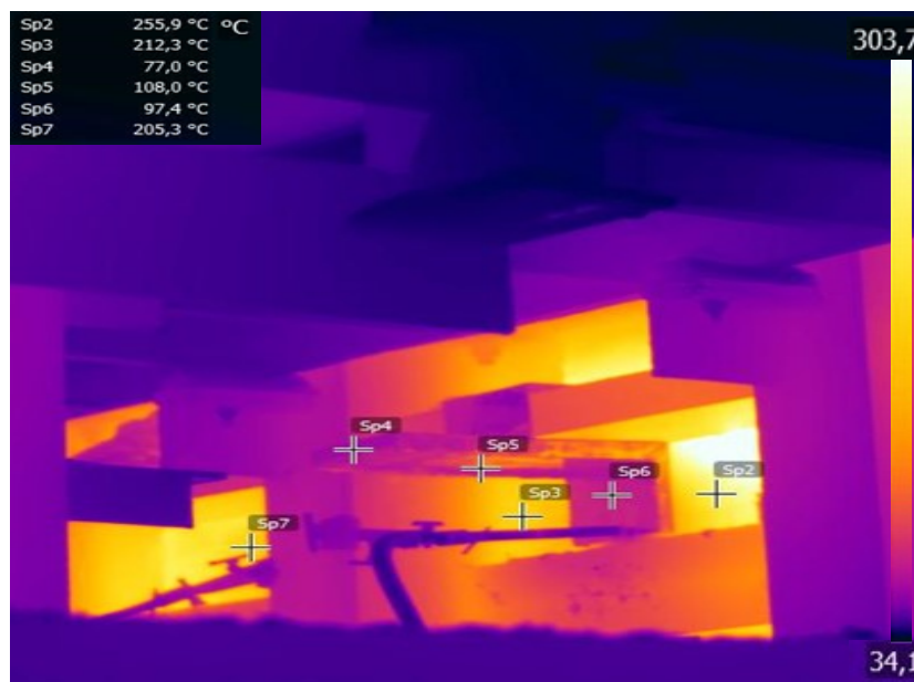
Figure 10. Reduction pot sidewall thermal profile picture.
